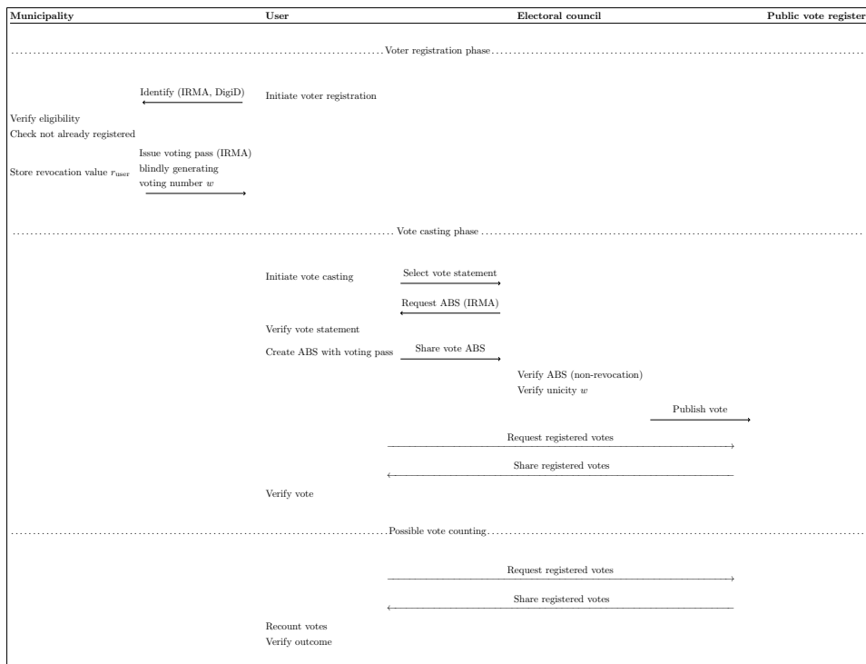
Scheme 4.4: Simplified overview of the voting scheme, based on blind voting number generation as proposed in subsection 4.3.4.
